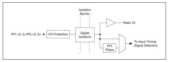
Figure 8-1. NI 6232/6233 PFI Input Circuitry
